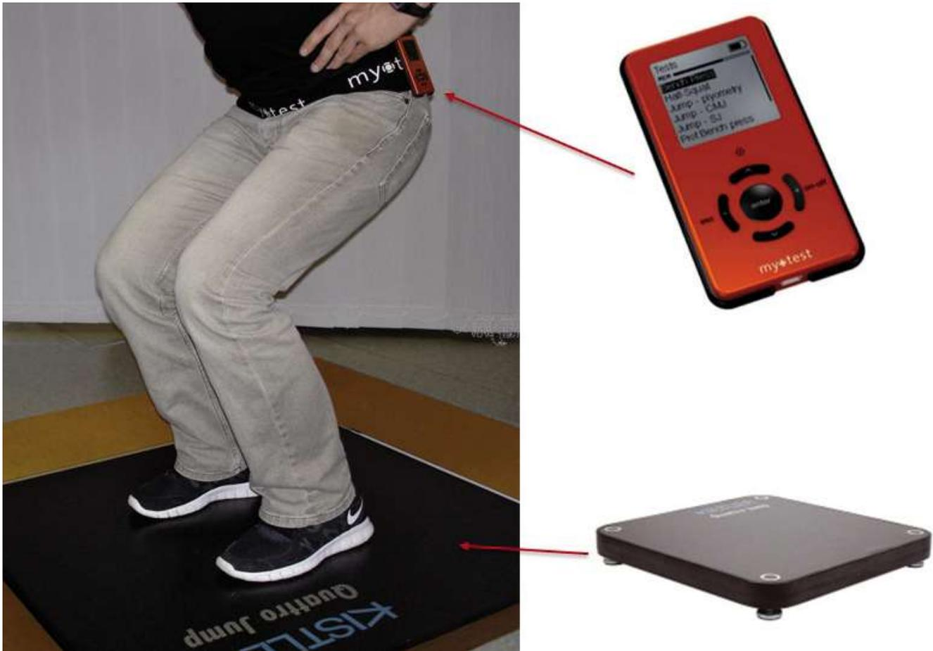
Figure 1: Squat jump. Simultaneous measurement with Myotest and Quattro Jump.
