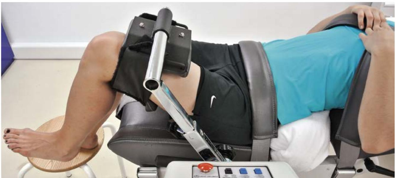
**Figure 2:** Test settings for the evaluation of hip flexor strength using an isokinetic dynamometer.
